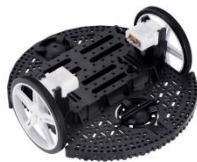
Chassis & Motor assembly with encoder
