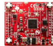
SimpleLink Wi-Fi® CC3100 wireless network processor BoosterPack plug-in module
