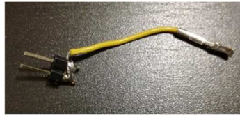
Figure 9: AD8232 GND pin and HC-06 GND pin connections in case of no soldering option
