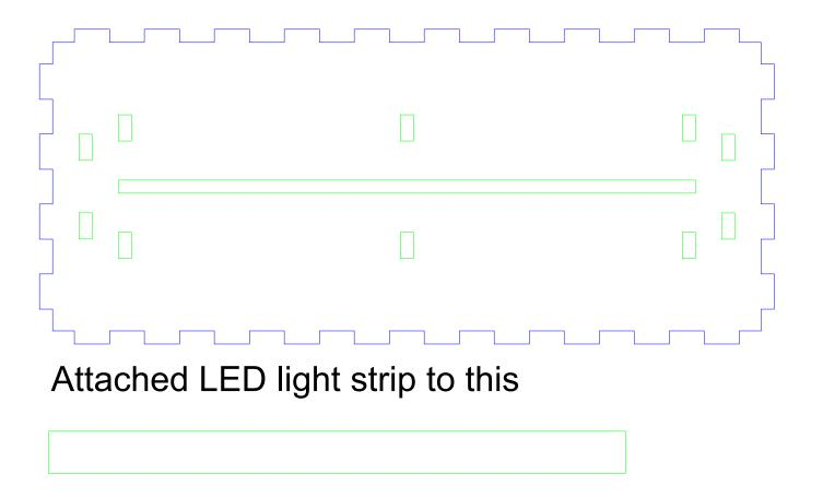
These hold the above LED strip holder directly under the slot for the acrylic
