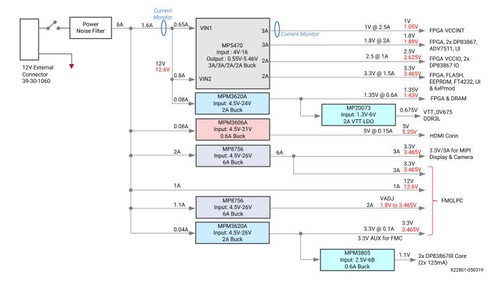
Figure 21: Power System Block Diagram
