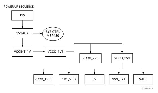
The options for VADJ are 1.8V, 2.5V, and 3.3V. They can be selected using the System Controller (MSP430) I2C connected TCA64164A I/O expander U24 ports P06 VSEL0\_VADJ and P07 VSEL1\_VADJ pins. The VADJ regulator can similarly be powered ON/OFF by the TCA64164A I/O expander U24 port P04 pin.
