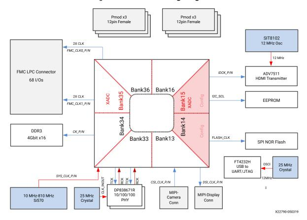
Figure 7: SP701 Clocking Diagram
