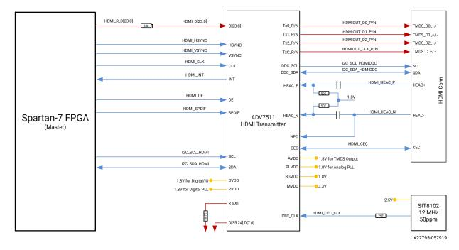
Figure 13: HDMI Output Interface
