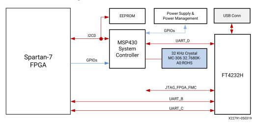
Figure 8: FTDI USB UART Circuit
