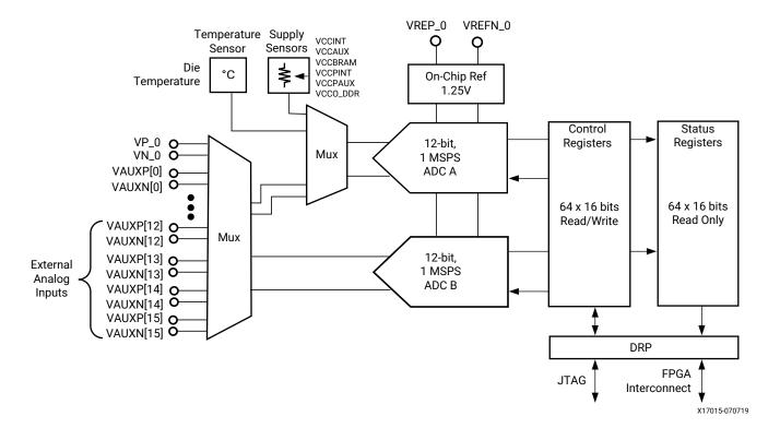
Figure 23: XADC (SYSMON) Block Diagram
