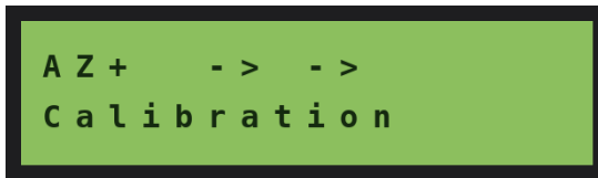
Calibrating azimuth clockwise (each leg is labeled: AZ+, AZ-, EL+, EL-)
