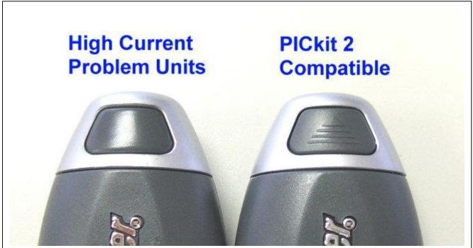
**Note:** The Energizer Energi To Go product pulses the USB voltage output to detect a connected device, as shown below. This may cause the PICkit 2's internal microcontroller to improperly reset, as its Brown Out Reset (BOR) is not enabled. The BOR is not enabled because it interferes with PICkit 2 VDD error detection.
