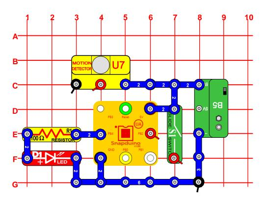
OBJECTIVE: This experiment will demonstrate the how to detect motion using the Snapduino.
