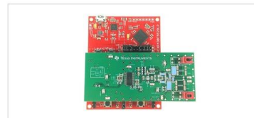
TIPD188 - High-Resolution, Low-Drift, Precision Weigh-Scale Reference Design with AC Bridge Excitation
