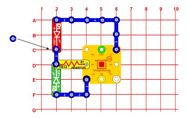
OBJECTIVE: This experiment will demonstrate how to control two LEDs using a single output pin on the Snapduino.
