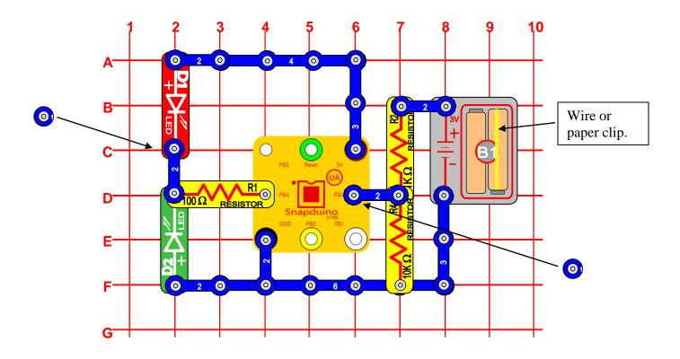
OBJECTIVE: This experiment will use the Snapduino to create device that can test the condition of a AA battery.
