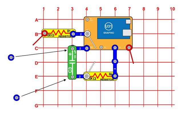
OBJECTIVE: This experiment will demonstrate the Arduino **Capacitance Meter and RC Time Constants** project found at https://www.arduino.cc/en/Tutorial/CapacitanceMeter.
