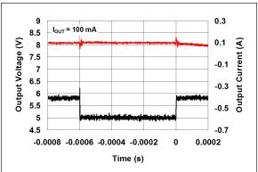
**FIGURE 2-20:** Line Transient Response.  $I_{OUT} = 100 \text{ mA}.$
