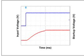
FIGURE 2-25: Startup Delay.
