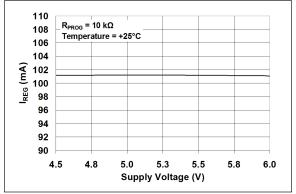
**FIGURE 2-10:** Charge Current ( $I_{OUT}$ ) vs. Supply Voltage ( $V_{DD}$ ).
