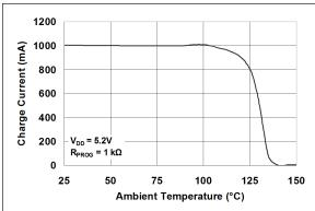
**FIGURE 2-14:** Charge Current  $(I_{OUT})$  vs. Junction Temperature  $(T_{ij})$ .
