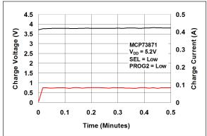
**FIGURE 2-26:** Complete Charge Cycle (130 mAh Li-lon Battery).
