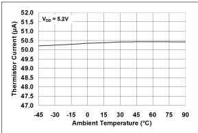
**FIGURE 2-18:** Thermistor Current ( $I_{THERM}$ ) vs. Ambient Temperature ( $T_A$ ).
