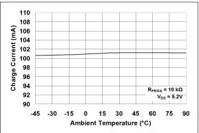
**FIGURE 2-12:** Charge Current  $(I_{OUT})$  vs. Ambient Temperature  $(T_A)$ .
