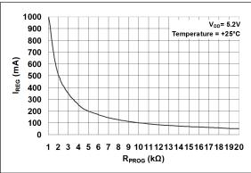
**FIGURE 2-3:** Charge Current ( $I_{OUT}$ ) vs. Programming Resistor ( $R_{PROG}$ ).
