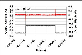
FIGURE 2-23: Load Transient Response. I<sub>OUT</sub> = 500 mA.
