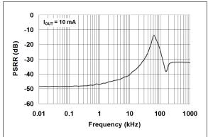
FIGURE 2-19: Power Supply Ripple Rejection (PSRR).
