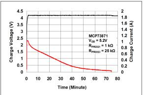
FIGURE 2-27: Complete Charge Cycle (1000 mAh Li-lon Battery).
