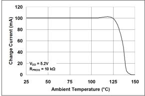
**FIGURE 2-16:** Charge Current ( $I_{OUT}$ ) vs. Junction Temperature ( $T_{J}$ ).
