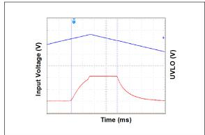
FIGURE 2-24: Undervoltage Lockout.
