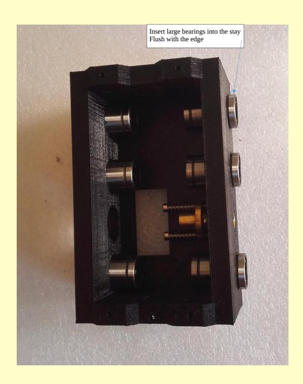
M3X12/6PCS Do not tighten very hard, just sufficiently to secure the bearing
