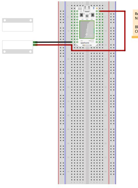
Red lead to 3v3 and NC side of switch
