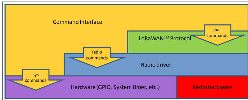
The available commands can be used to configure and control the LoRaWAN protocol layer, the radio driver and some system peripherals.
