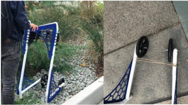
Figure 7. (left) Testing the high-fidelity prototype on rocks. (right) Attachment to prevent wheels from moving out of place.
