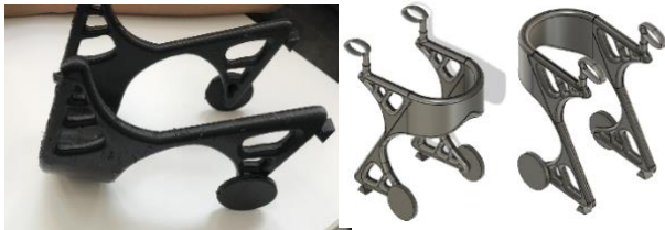
Figure 4. (Left) Low fidelity 3D printed model showing front loaded behavior. (Right) CAD model from two different views.
