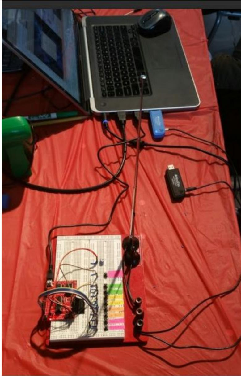
Figure 2 - Overview of system. The breadboard contains the radio user's interface, and the MSP launchpad which interprets the user's input and transmits the data to the PC. The PC runs the python code which controls the SDR dongle (blue USB stick), which receives the RF signals (via the antenna setup on the breadboard).
