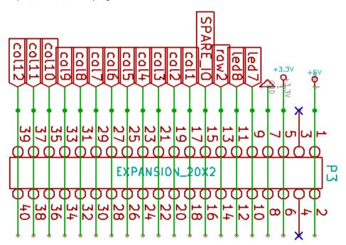
One obvious idea is to attach a spacewar controller/joystick to the expansion port. Look at gpio.c to understand how you can reach the in/output signals from software.
