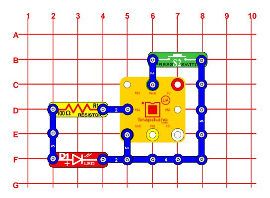
OBJECTIVE: This experiment will demonstrate the basic operation of the Snapduino by blinking the LED D1.
