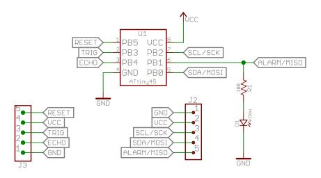
HC-SR04 sensor interface will be managed by the the ATtiny45 microcontroller, which will send the distance readings in centimeters each time they are requested by the I2C Master.
