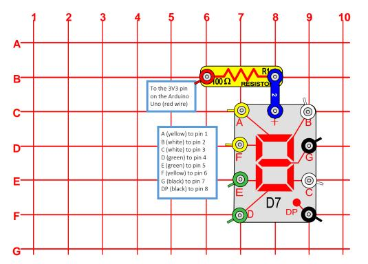
OBJECTIVE: Count from 0 to 9 on a seven segment display.
